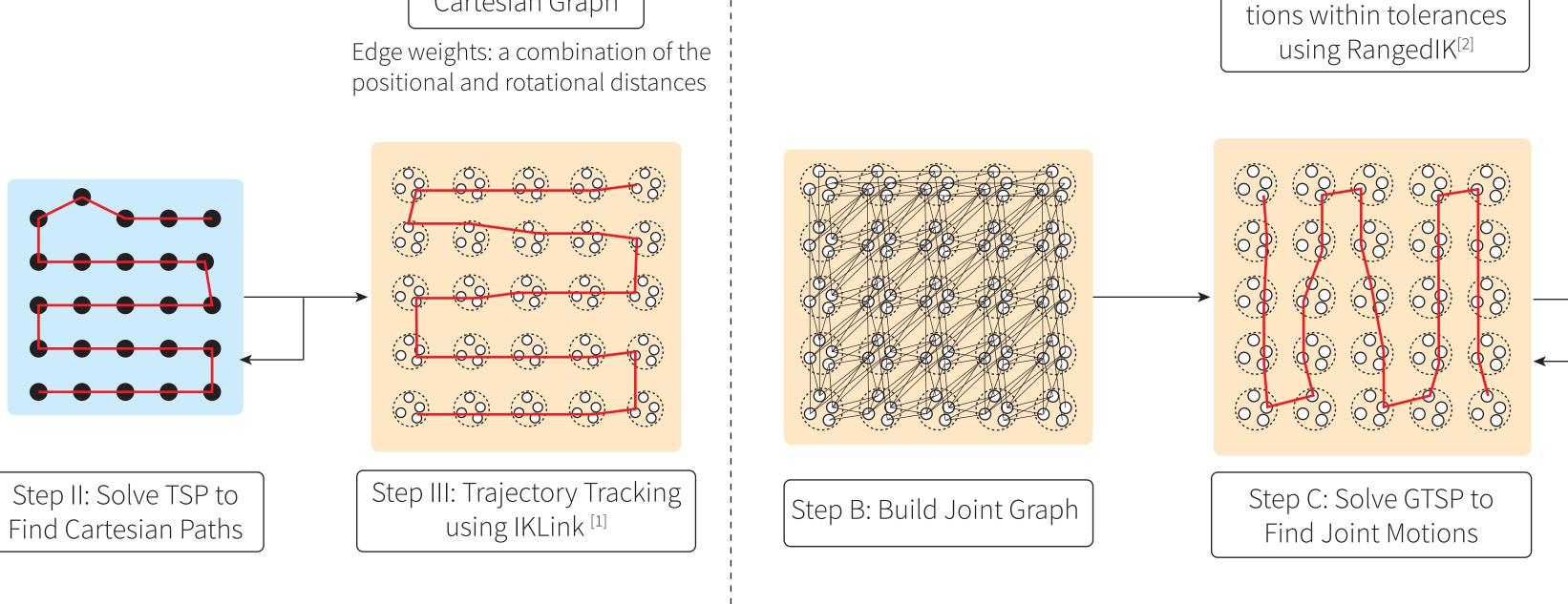
This method is efficient but plans in Cartesian space and can not achieve joint space objectives such as minimizing joint movements
